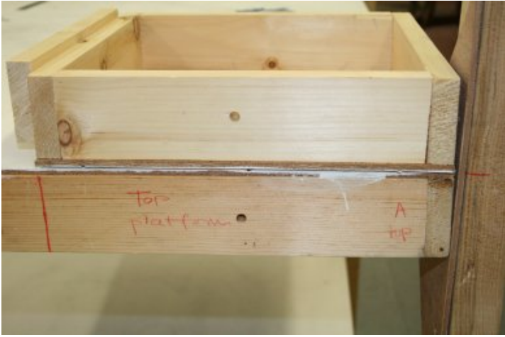
This piece is bolted to the upper platform in the position marked.
