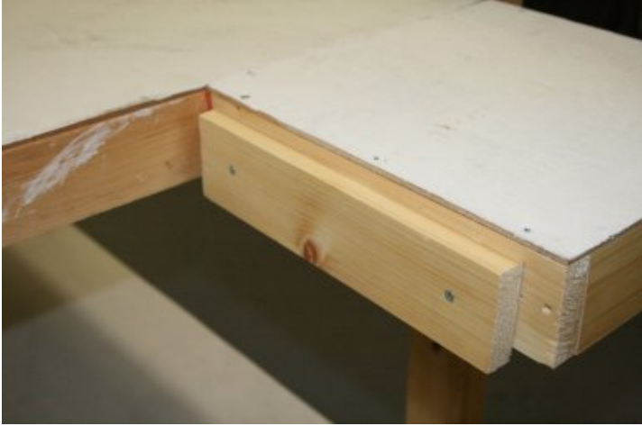
This piece is bolted to the upper platform in the position marked.
