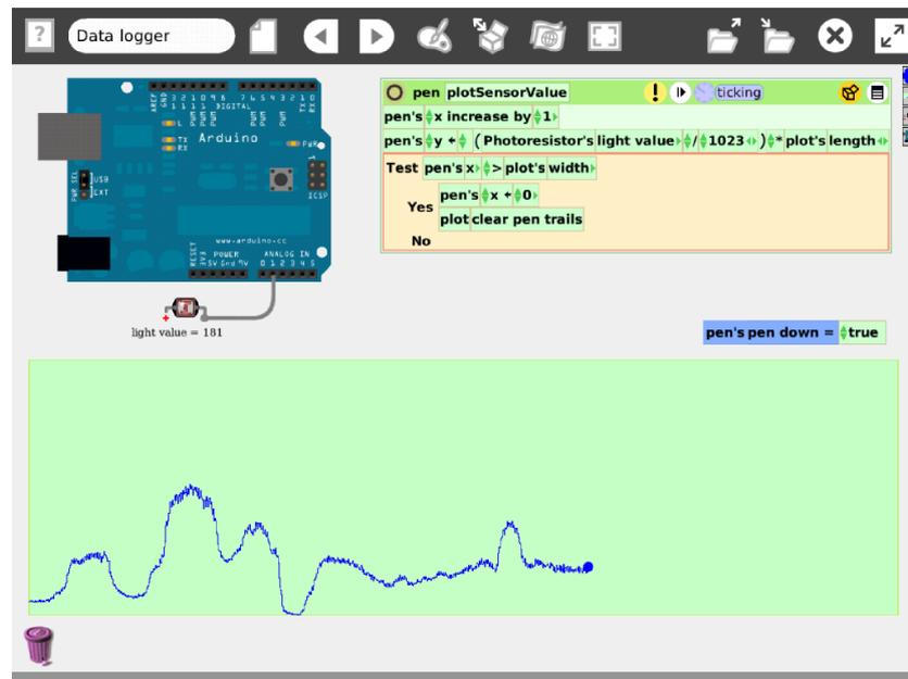
Fig. 1. Example of the “Direct” mode using an Arduino board as a data logger.
