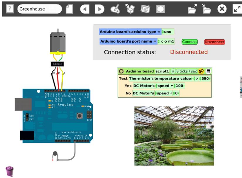
Fig. 2. Example of an Arduino board controlling the temperature of a greenhouse.
