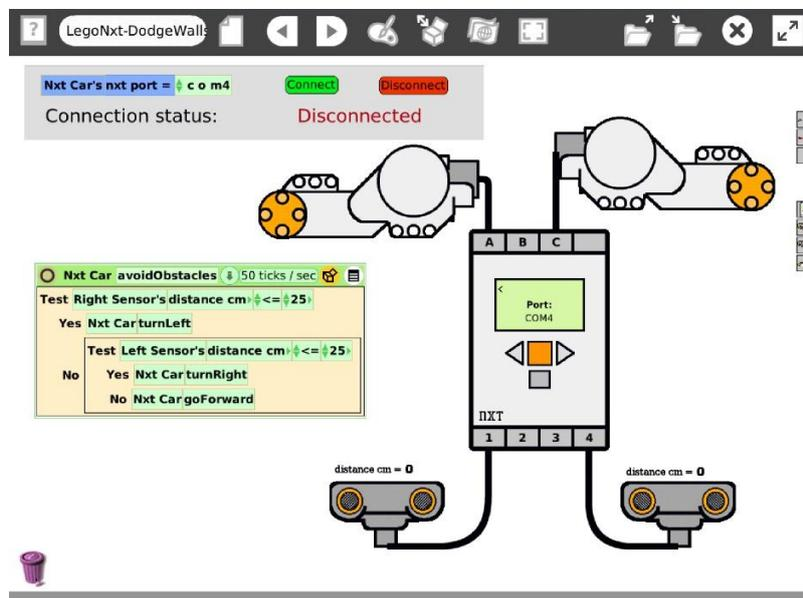
Fig. 3. Example of a simple autonomous robot built with Lego Mindstorms NXT that avoids colliding with walls.
