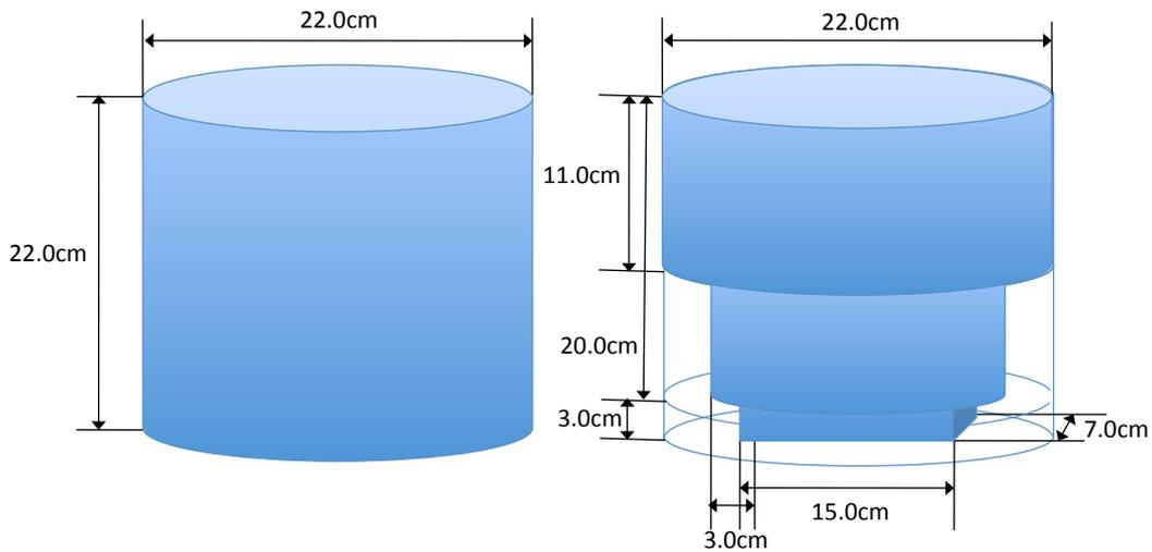
Fig.2 Size/Proportion of the robot for new rule
