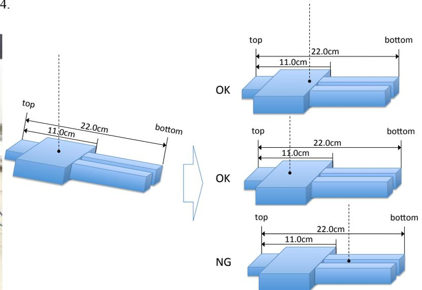
Fig.4 Limitation of the center of the gravity
